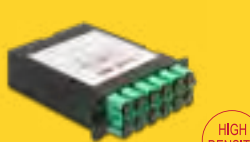
66936 Fiber Optic HD Cassette MPO male to 12 x SC Simplex female
