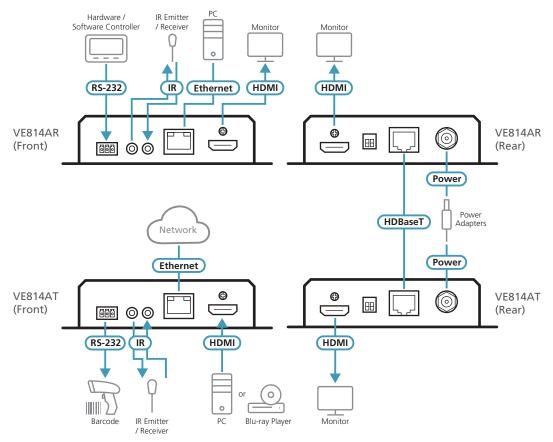
\* The Ethernet port is functional for device supporting the Ethernet port only.
