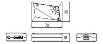
Note: The transmitter, DPFX-100-T and the receiver, DPFX-100-R have the same mechanical dimensions
