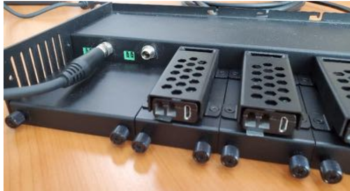
Fig. 6: Mounting the Module bracket on BR-500.
