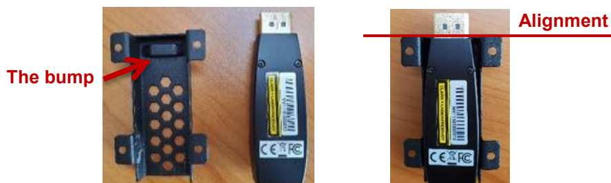
Fig. 2: Insert the push button into the bracket
