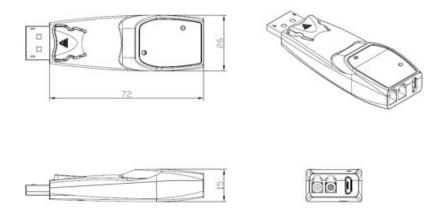
Note: The transmitter, DPFX-250-T and the receiver, DPFX-250-R have the same mechanical dimensions
