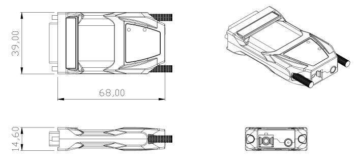
Note: The transmitter, DVFX-110-T and the receiver, DVFX-110-R have the same mechanical dimensions.
