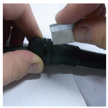
Use the knife to cut open the inner heat shrink tube, then the protection tube and the gland divide.
