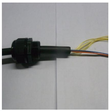
Drop out the protection tube from the fan-out carefully
