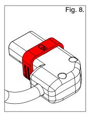
Replace the cord grip (Fig. 7.) ensuring the torque value is achieved (0.3Nm), and then replace the outer housing, screws and handle (Fig. 8.).
