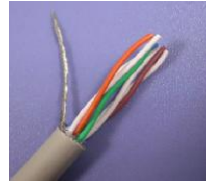
3. Cut foil for 4 Pair Wires
