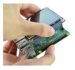
**NOTE:** The 4DPi-24-HAT is supported only by the 40 way header, and therefore pressing on the touch screen may result in the 4DPi-24-HAT moving towards the Raspberry Pi, and therefore the circuitry touching the Raspberry Pi. This could result in damage to either product if a short circuit were to occur. It is therefore highly encouraged to mount the display on the Pi using standoffs (not supplied). Some options are available from places like Mouser.
